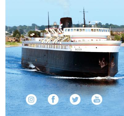
The 410' sister ships, S.S. Spartan and S.S. Badger, launched in 1952 and 1953, were the last — and largest — coal-fired, steam engine car ferries built in the United States.
